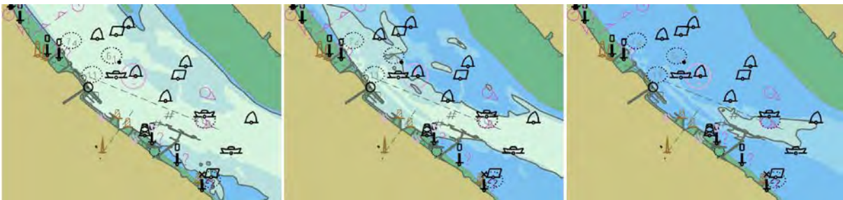
Figure 2. The water area outside Immingham oil terminal in an electronic chart. The safety contour is set to 2 (left), 5 (middle), and 10 meters (right). The contours need to be present in the chart database, so, for instance, a safety contour of 8.5 meters cannot be set: it will instead be the next deeper contour, 10 meters.
