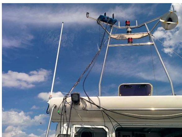
Figure 5 Installation of the antennas on the ship during the Seamless Roaming on-board tests
