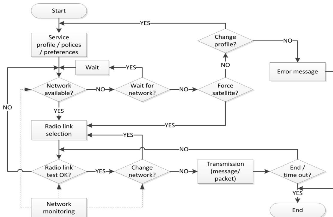
Fig. 18. General algorithm of the Seamless Roaming mechanism
