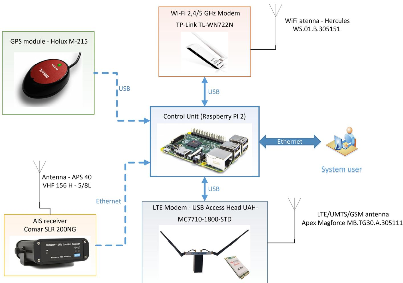
Fig. 3 Proposed hardware architecture of the onboard module
