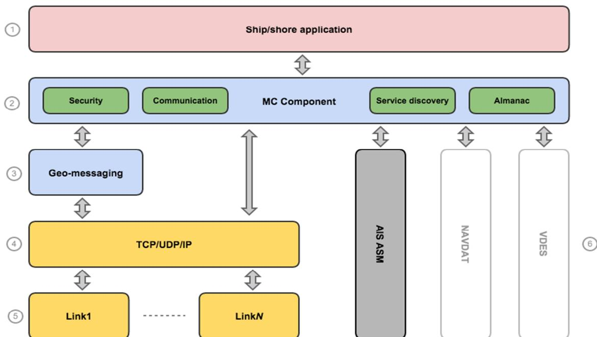
Fig. 15. The Maritime Cloud client component shown as a layer of the OSI model [8]
