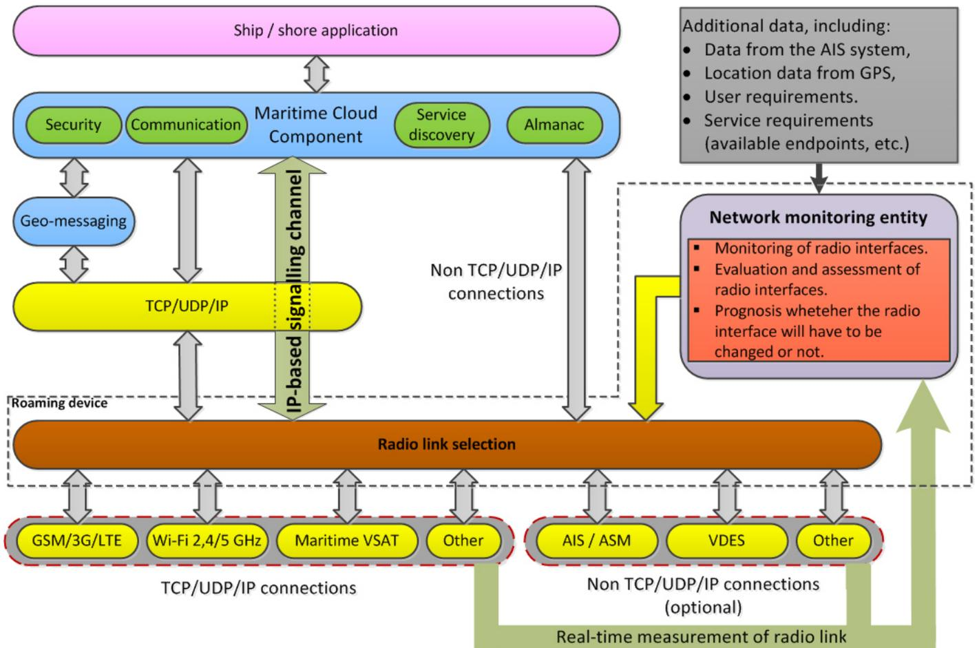
Fig. 16. The architecture of the Maritime Cloud client connected with the components of the hybrid communication system and the Seamless Roaming
