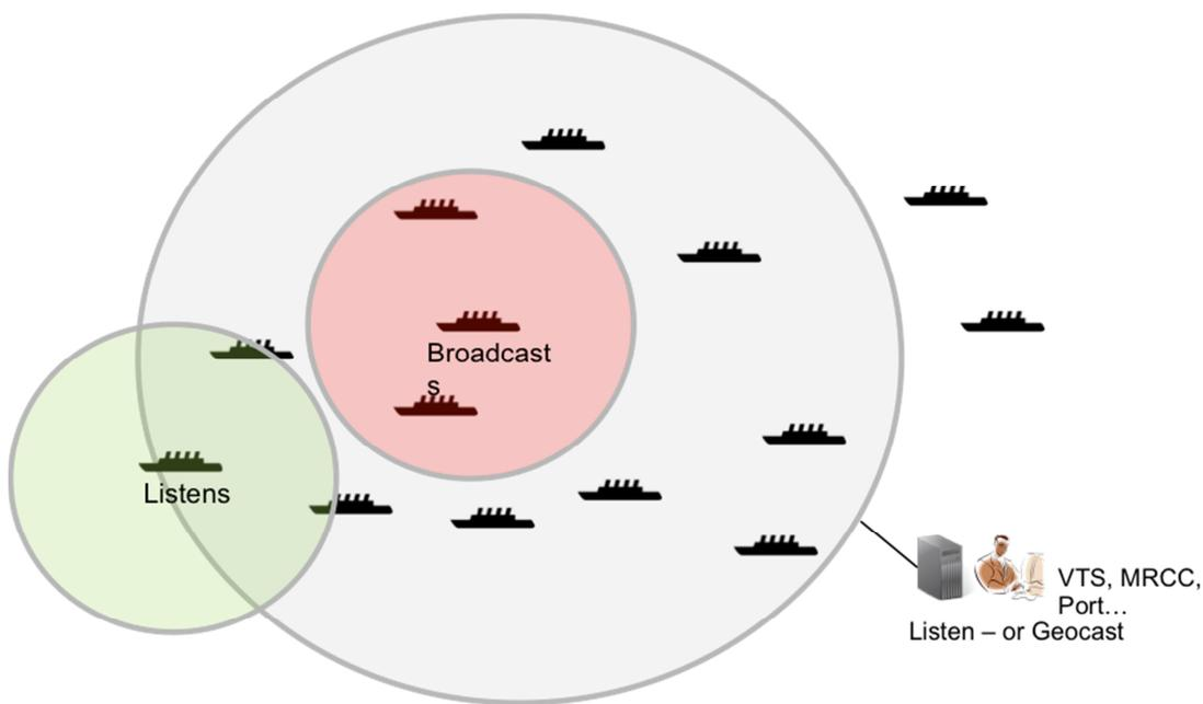
Fig. 14. General concept of geocasting [8].
