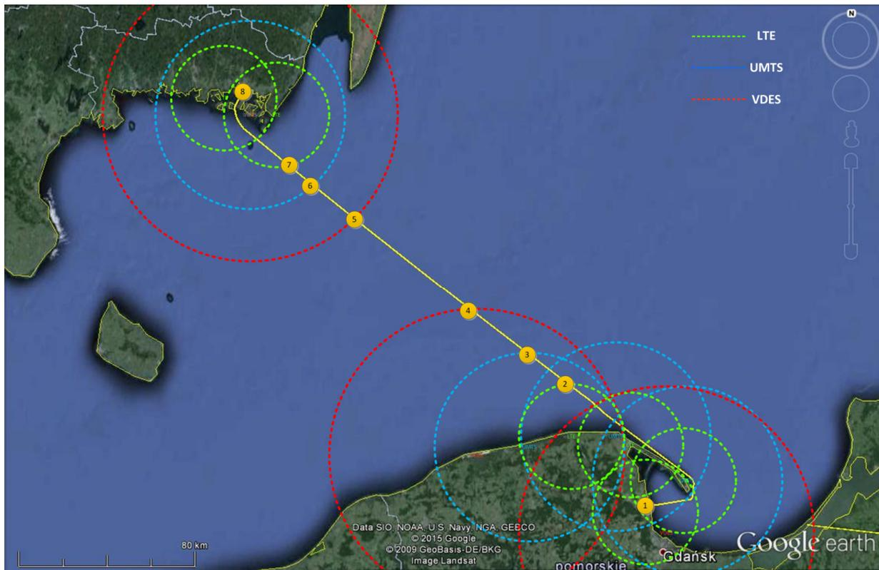
Fig. 20. Approximate ranges of the terrestrial radiocommunication systems along the ferry route from Gdynia to Karlskrona.
