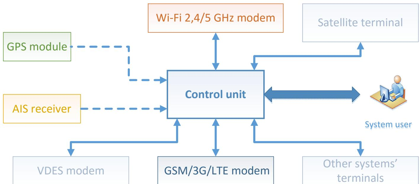
Fig. 2. General architecture of the onboard module.
