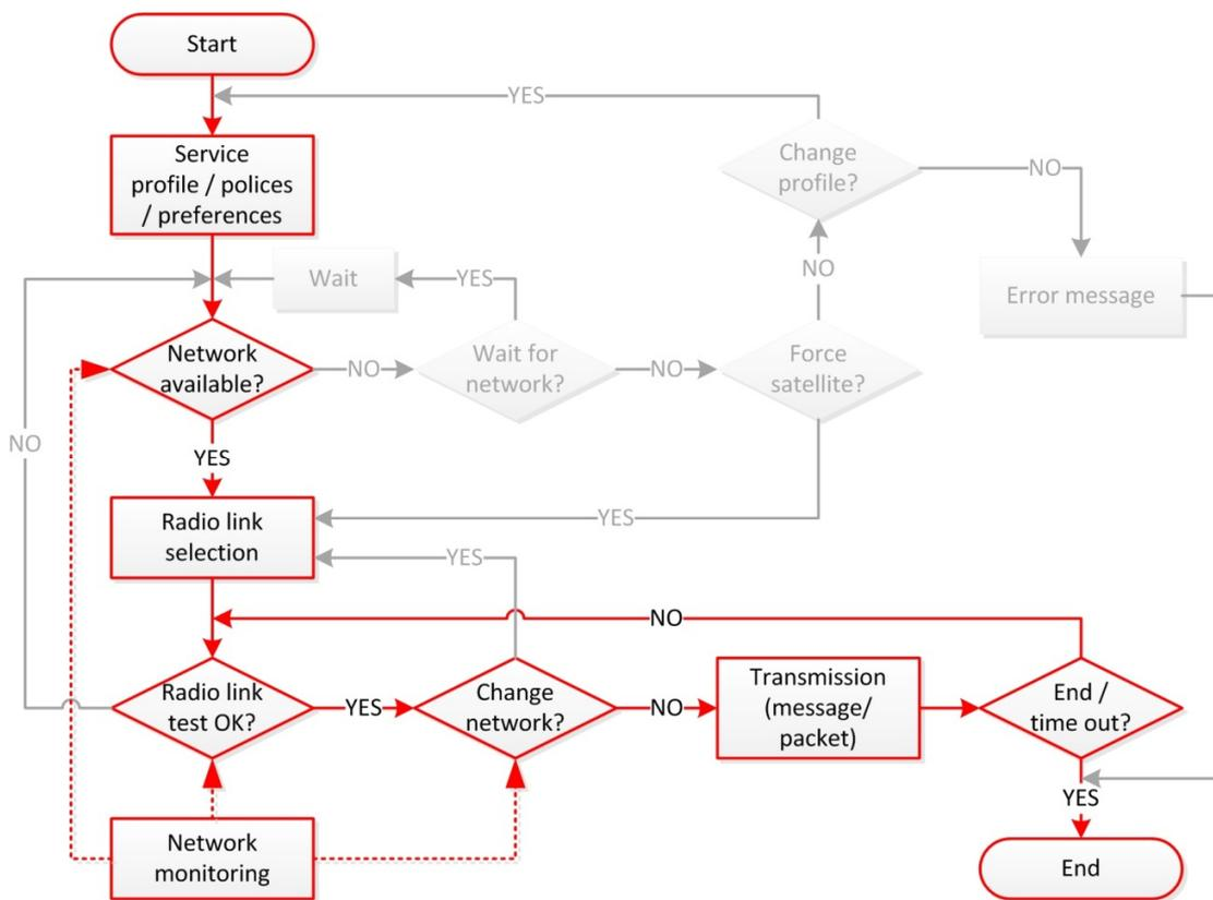
Fig. 19. An example of the Seamless Roaming mechanism
