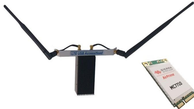
Fig. 8. LTE USB Access Head UAH-MC7710 module and AirPrime MC7710 LTE/HSPA+ card.
