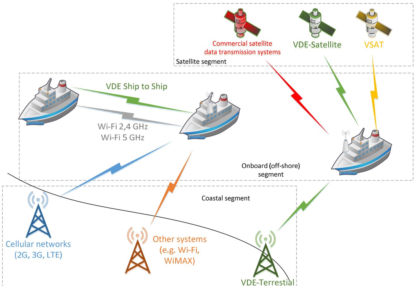
Fig. 1. The architecture of the hybrid communication system.
