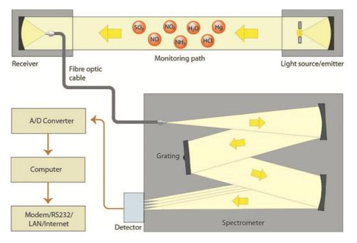
Figure 10: Diagram of the DOAS principle<sup>24</sup>
