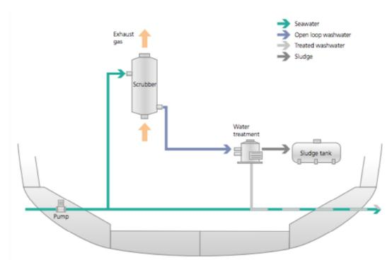
Figure 5: Process diagram of an open-loop scrubber installation<sup>11</sup>
