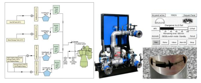
Figure 11: On the left, diagram of typical vessel fuel supply. On the right, fuel oil change over system by LEMAG<sup>27</sup>
