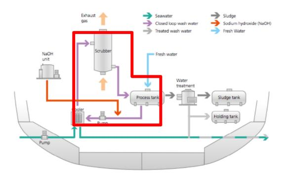
Figure 6: Process diagram of a closed-loop scrubber installation<sup>12</sup>
