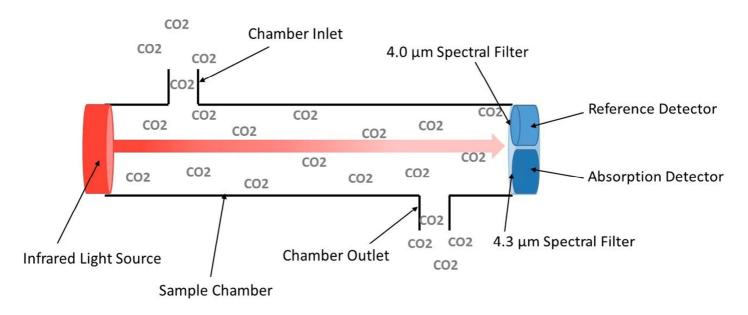
Figure 7: Principle of extractive NDIR spectrometer<sup>15</sup>
