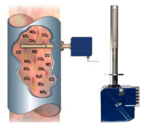
Figure 9: On the left placement of Procal2000 SOx sensor, on the right the Procal2000 sensor<sup>22</sup>
