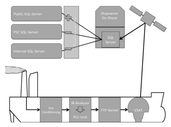
Figure 14: Flowchart of extractive CEMS with cloud solution
