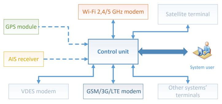
Fig. 2. General architecture of the onboard module.
