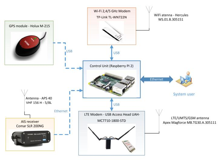
Fig. 3 Proposed hardware architecture of the onboard module
