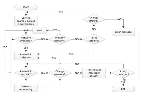
Fig. 18. General algorithm of the Seamless Roaming mechanism
