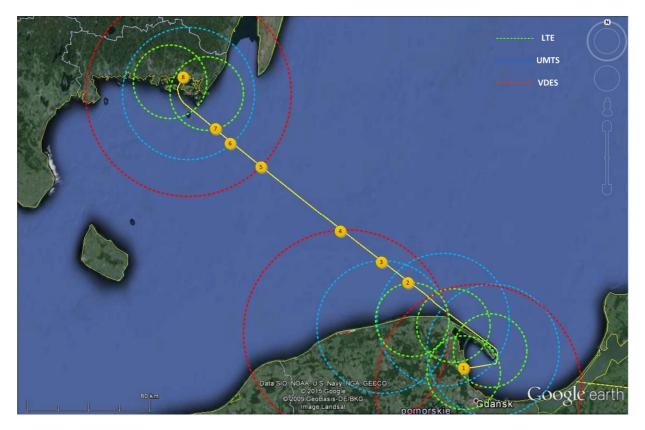
Fig. 20. Approximate ranges of the terrestrial radiocommunication systems along the ferry route from Gdynia to Karlskrona.
