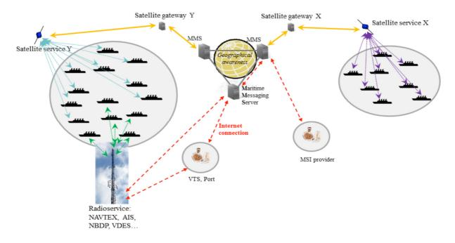
Fig. 13. General concept of the MMS service in the Maritime Cloud [8].
