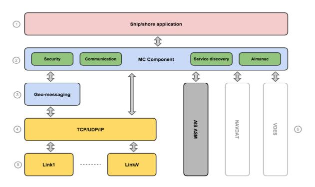
Fig. 15. The Maritime Cloud client component shown as a layer of the OSI model [8]
