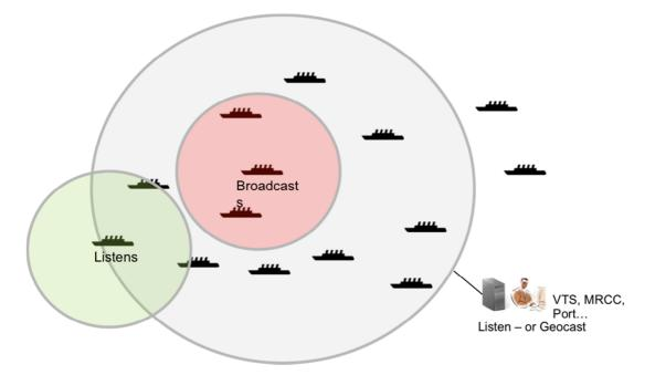
Fig. 14. General concept of geocasting [8].
